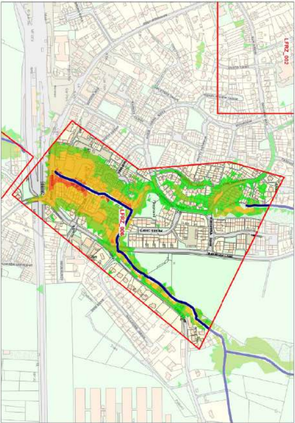
Figure 7.14 - Flood Hazard LFRRZ_006 (1 in 100 year storm event)
