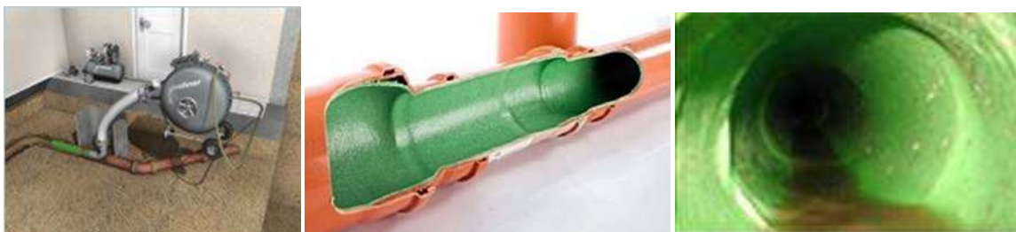
Figure 10.17 - Overview of Sewer Relining
