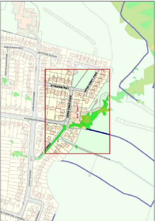
Figure 7.34 - Flood Hazard LFRRZ_016 (1 in 100 year storm event)
